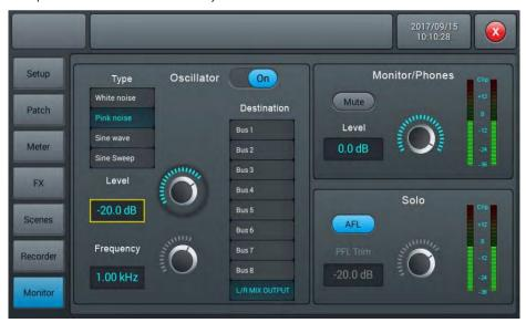
Set up your microphone at least several meters away from the speakers to pick up their full range. Ideally put it in the center position of the audience. Turn up the master fader sending pink noise to your system until your microphone clearly picks up the audio on the level meter of your microphone channel.
