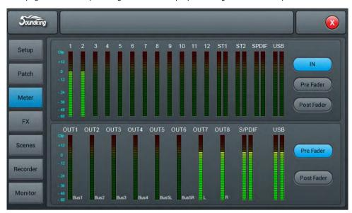
Signal level of input processing channel has three modes IN, Pre Fader and Post Fader with Pre Fader as the default. To select signal level mode to be displayed through single pressing the button. The signal level of output has two modesPre Fader and Post Fader with Pre Fader as the default. To select signal level mode to be displayed through single pressing the button. On the right side of signal level of outputs you can see the bus names which are assigned to the port.
