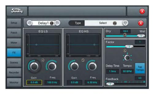
The Effects have 8 modules, which are 2 Modulation, 2 Delay, 2 Reverb and 2 15-band GEQ. All the modules can be inserted to input processing channel or bus processing channel, for one time only. Note, input processing channel can only be inserted with one effect module, while the bus can have two.
